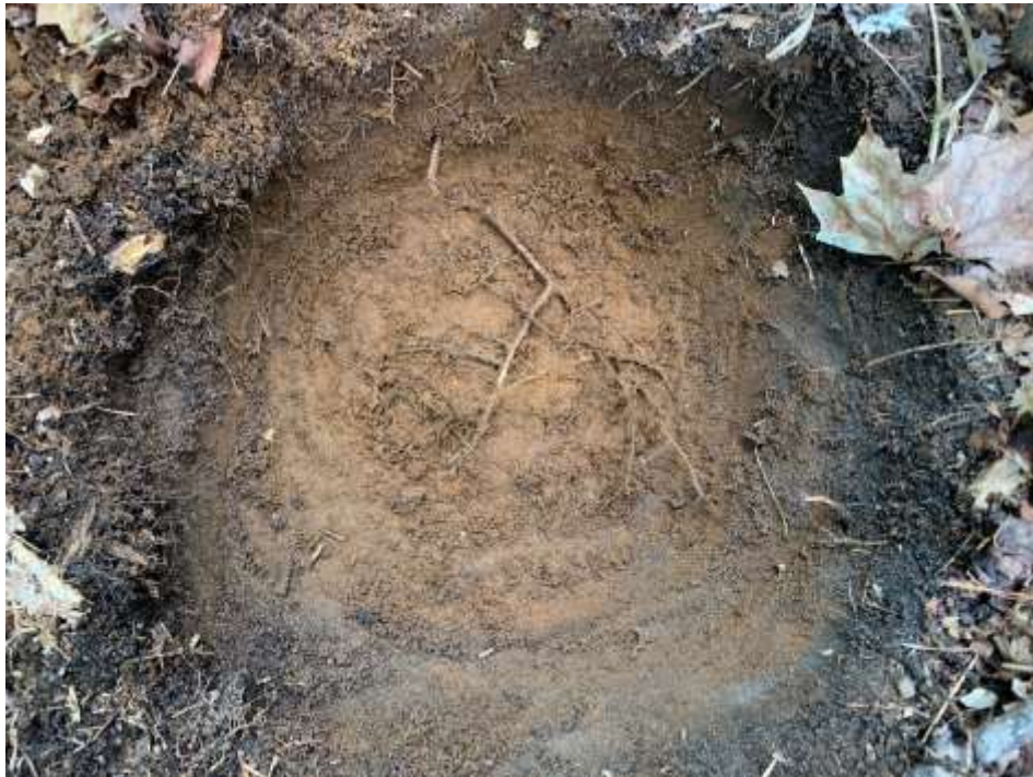
Image 46: Open Test Pit showing Subsurface Stratigraphy.
